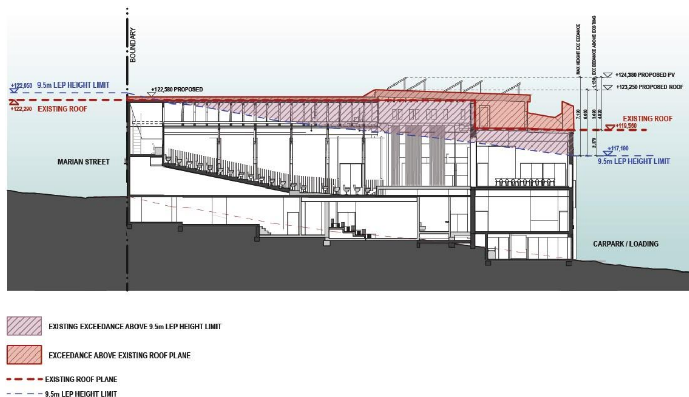
Figure 4 Section showing height exceedance over the LEP and existing roof plane
