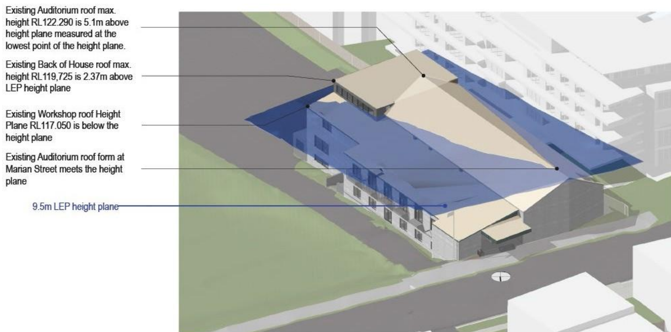
Figure 2 Height plane diagram showing extent of the existing non-compliance with the height control
